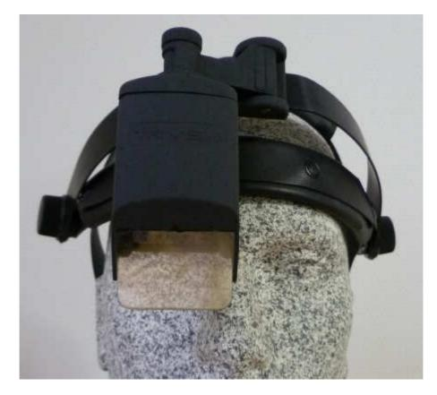
The M3 Monocular HMD is a specialized product designed for Augmented Reality applications. It is a monocular optic-see-through device that projects an image or a streaming video through the near-the-eye micro-display. The frameless design allows nearly unblocked vision.
